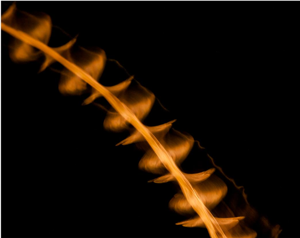
**FIGURE 10.** An insect flight trace using incandescent light only. The broad portions of the trace are created during the insect's downstroke. The upstrokes are narrow peaks between the downstrokes. Note orange colour of trace caused by reduced voltage from power drain on battery.
