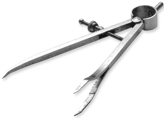
FIGURE 2. Metal grab used to clamp P. lividus and measure attachment force when connected by a hook to a spring dynamometer. The gear consists of a steel compass modified as a grabbing claw that allows a proper grip to sea urchins even when inside tight burrows.
