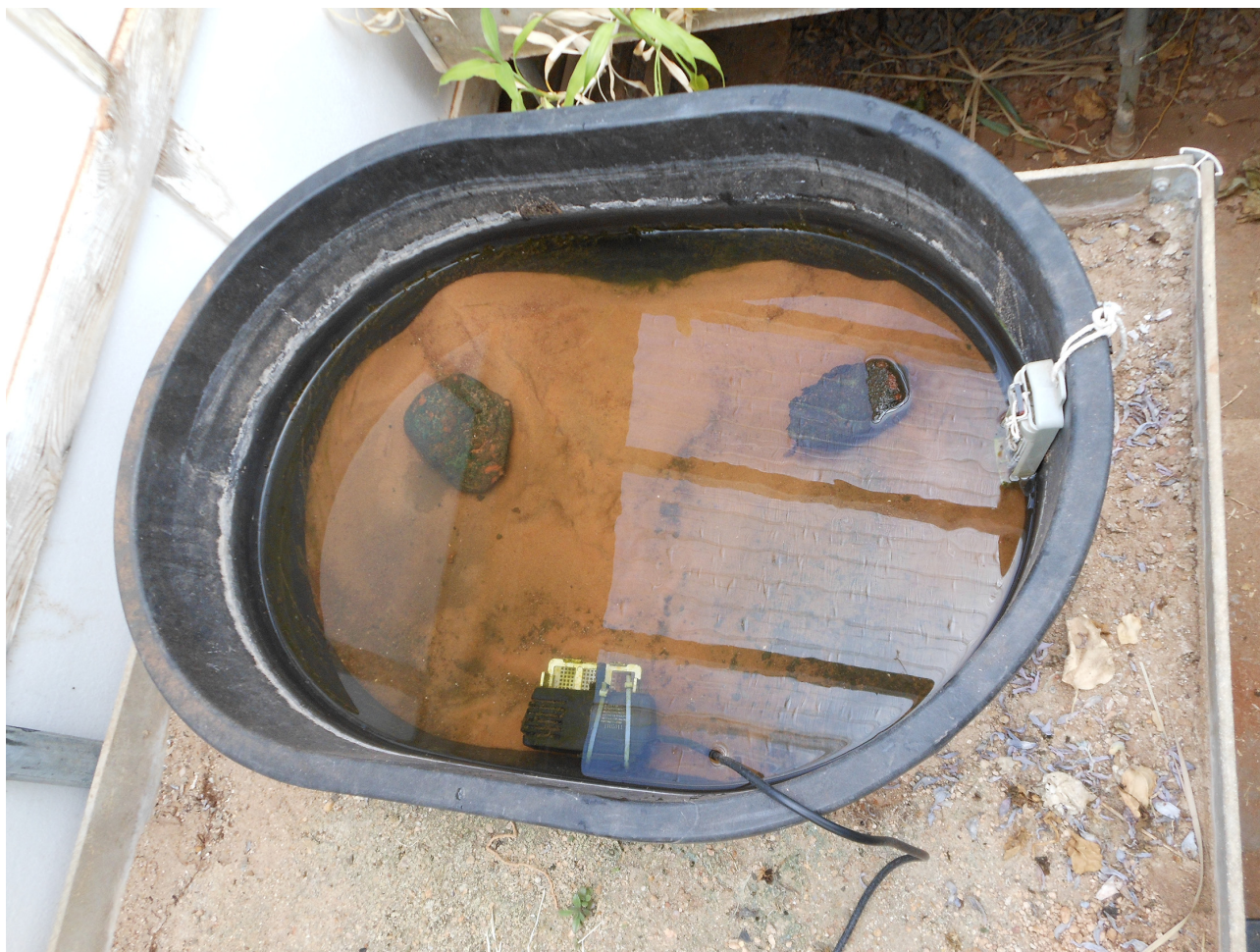
FIGURE 1. Overhead view of artificial stream. Pump is in the tub on the bottom of the photo (connected to electrical cord). Two large, dark stones rest on the sandy substrate. A maximum-minimum thermometer is to the right.
