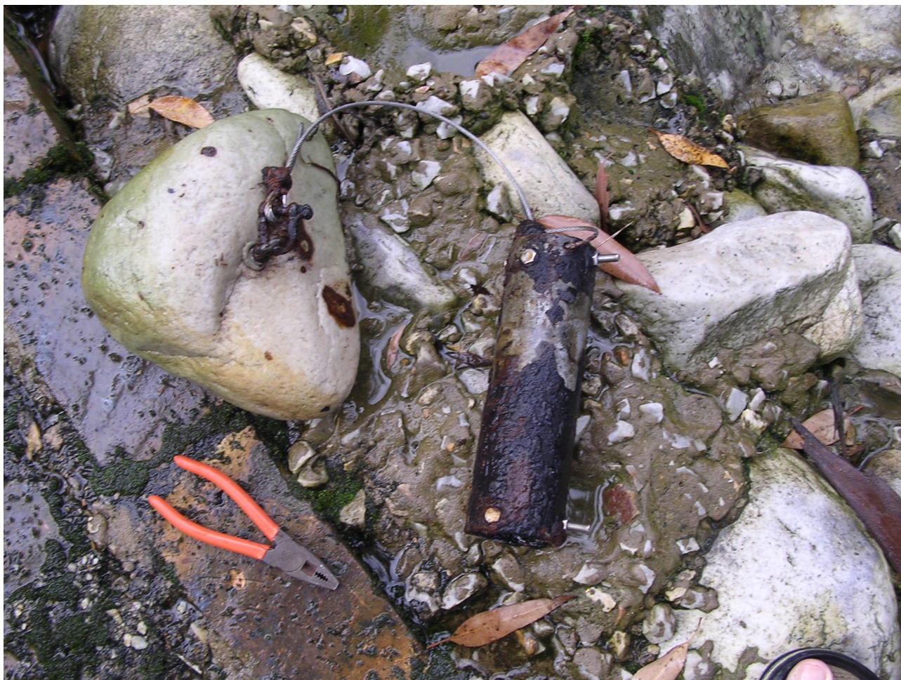
FIGURE 2. Boulder with stainless steel cable attached to galvanised pipe, with ends sealed by stainless steel nuts and bolts, used for storing Thermocron temperature recording i-buttons in plastic containers under water for extended time.
