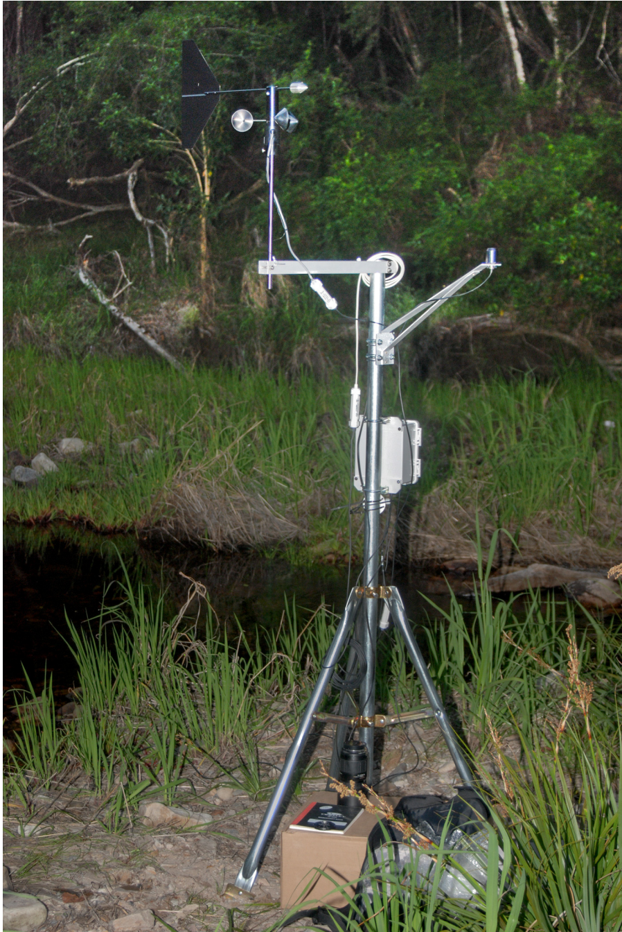
FIGURE 3. Onset HOBOWare® Weather Station set up to capture data at study site on Groot River.
