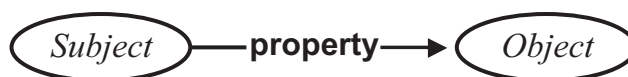
FIGURE 2. A RDF triple modeled as a directed labeled graph (DLG). Subject and Object represent the nodes and the ' property ' the edge that connects the nodes.
