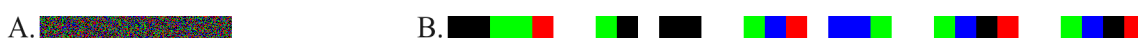
FIGURE 6. A. Ten thousand base pair sequence coded as a 4-color 2D barcode, printed at 300 dpi (printed matter resolution for Zootaxa ). Color codes according to the RGB color space, as in electropherogram colors, as follows: A = green (RGB 0,255,0), C = blue (RGB 0,0,255), G = black (RGB 0,0,0) and T = red (RGB = 255,0,0). B. Diagram showing pixel-level encoding for GGAATRGGHCCANN. Note that R = either A/G, H = ACT ( i.e. , not G), and N = any base (ACGT).
