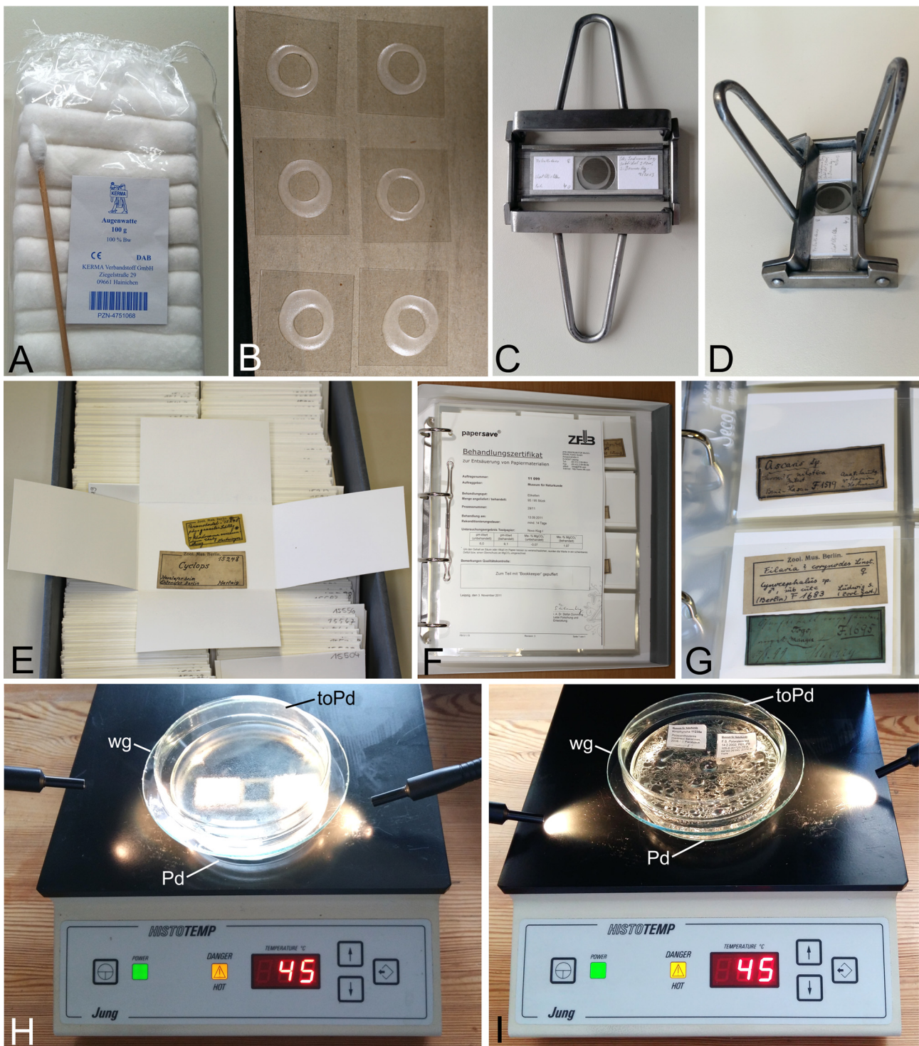
FIGURE 27. A. Absorbent purified cotton wool wrapped on skewer. B. Coverslips 24 mm x 24 mm with paraffin rings ready for mounting each specimen in a drop of glycerol on a Cobb aluminum slide. C, D. Slide mounting device for Cobb aluminum slides. E. Storage of labels in 4-flap paper envelopes filed in cardboard boxes provided by Klug Conservation. F, G. Storage of labels in Secol polyester slide and negative film preserver sheets housed in a custom-made cardboard file system made by Klug Conservation. Note certificate of deacidification with Bookkeeper™ in front of the labels ( F ) and sheet of paper behind labels in polyester envelope ( G ). H, I. Restoration of a microscope slide by soaking the slide in distilled water on a hot plate in the lower part of a Petri dish (Pd) covered with a watch glass (wg) before ( H ) and after removal of labels and their storage under the top of the Petri dish ( I , toPd). Note drops of water dripping back into lower Petri dish ( I ).
