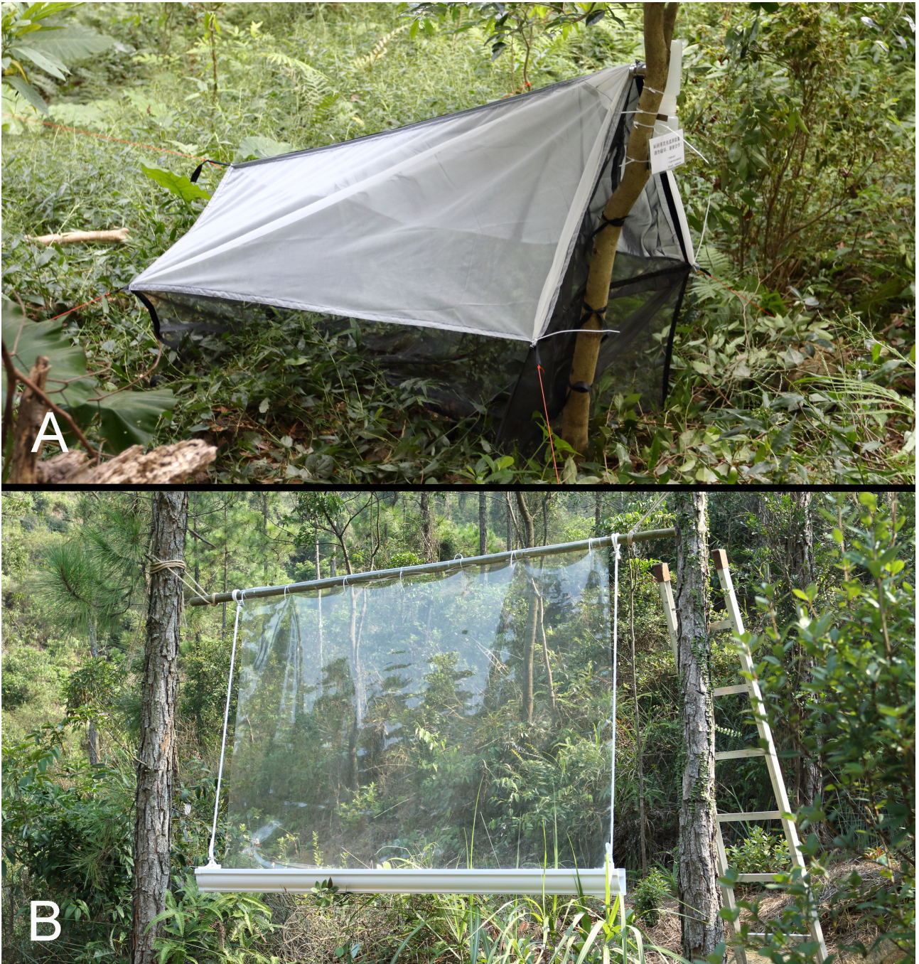
FIGURE 1. Examples of passive acquisition methods. A. Malaise trap. B. Flight intercept trap.
